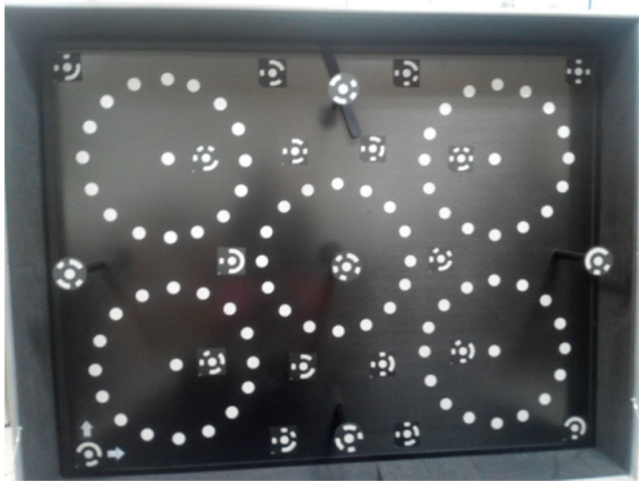
Fig. 4. AICON 3D Systems GmbH calibration board.
