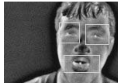
Figure 5: Example output of our interest point clustering approach for facial feature localization.
